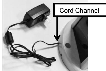
Step 4: Plug in the charger and let charge overnight. Wait a minimum of one hour and verify battery state-of-charge. The most accurate Battery Pack status reading is obtained when the lantern has been in a dark location and in “off” mode for at least 24 hours.
