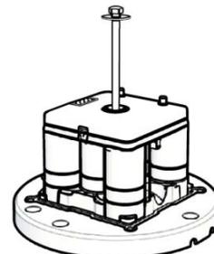
7. Lift out the battery pack. Remove the old black rubber gasket in the lantern base and replace it with the new one supplied.
