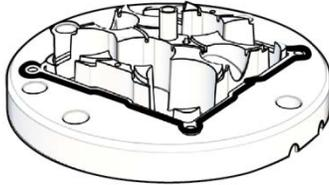
8. Position the replacement pack in the lantern base. Attach the new pack to the base using the centre bolt and washer. Torque centre bolt to 40 inch lbs.
