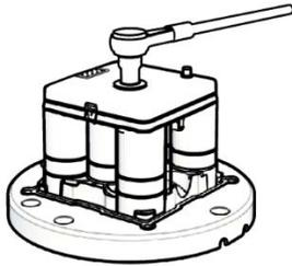
9. Place the lantern housing back over the battery pack and re-connect the battery harness.
