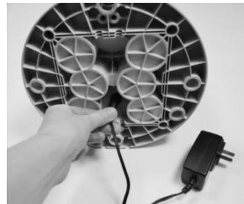
Step 3: Align the charger cord with the cord channel at the base of the lantern.
