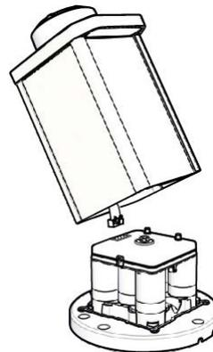
6. Using the ½" socket, remove the center bolt and washer.
