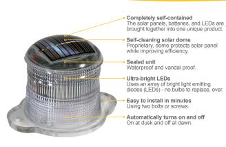
Carmanah's Model M502 solar marine lantern is a compact, lightweight, and low maintenance solution for marking small buoys, docks, marinas, aquaculture weirs, and other applications requiring navigation or hazard marking.
