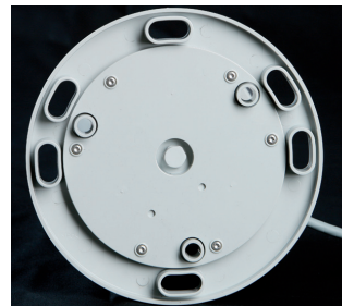
Installation The bottom plate of the LED110 supports installation on structure using 3 or 4 x M12 on a 200 mm diameter or 3 x M8 on a 150 mm diameter.
