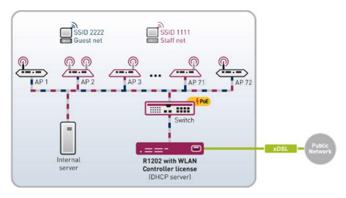
For 7 - 72 access points, the bintec Rxx02 series (e.g. R1202) hardware is required. To run it, you require a WLAN controller licence on a bintec router.
