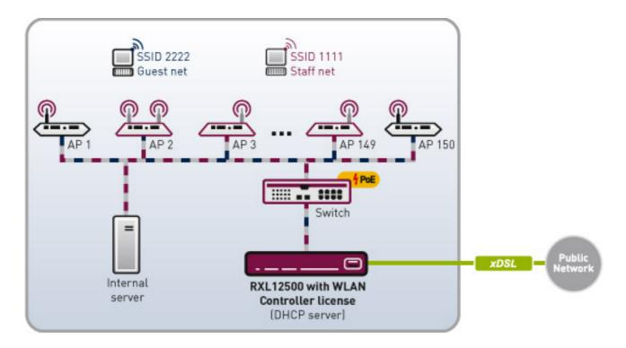
For 72 - 150 access points, a bintec RXL series hardware is required. To run it, you require a WLAN controller licence on RXL series.
