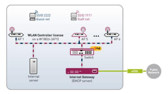
No additional hardware is required for the smallest version (up to 6 APs) because the WLAN controller software is run as a licence on a master access point.
