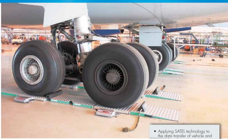
The benefits are clear. EVOPLANE makes measurements accurately, quickly and, above all, safely. Measurement personnel do not need to be near the aircraft during the process. Previously, weighing took place, for example, using three detectors at wing measurement points, which in terms of accuracy was uncertain, time consuming and awkward. A new, more precise version of EVOPLANE for weighing fighter jets is under development.
