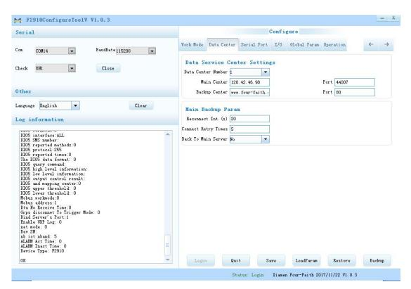
After Re-power NB-IoT Terminal, The configure tool will make it enter configure state. At the same time, the software will load current settings from NB-IoT Terminal and displays on the right configure columns at the same time.. It's now ready to configure.
