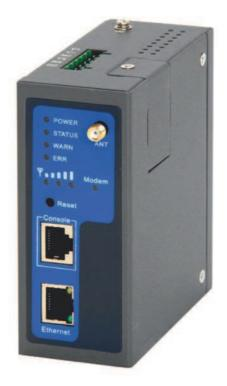
TK700 Series industrial grade routers provide users with stable and high speed connection between remote devices and customer's center via 2.5G/3G networks. They allow wide voltage power supply (9-48V DC), large range operating temperature from -25°C to 70°C (-10 ~ 158F)/ humidity: 95% RH, and fully satisfy various EMC verifications, which ensure stability and reliability under harsh industrial conditions. The TK700 can be placed on a desktop or DIN-mounted.
