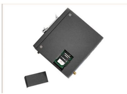
Open TK Router SIM/UIM card case at the button, insert the SIM card and close the case.
