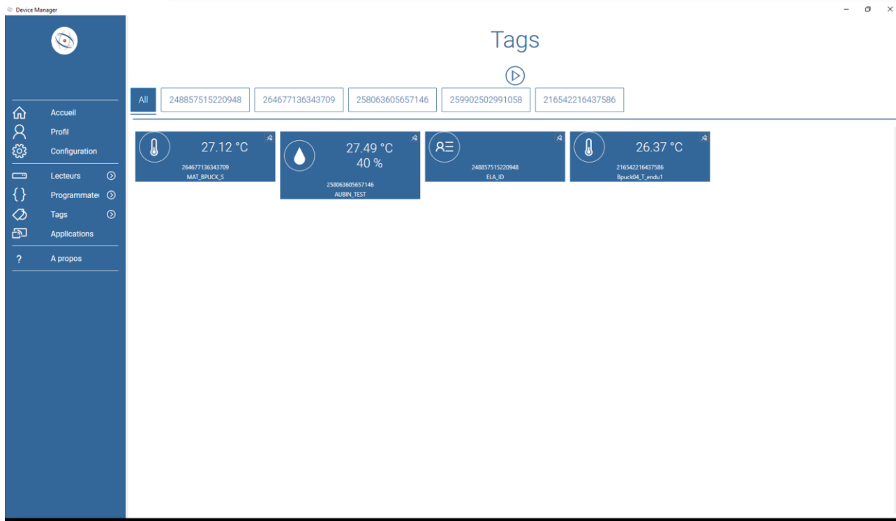
Figure 116 – Monitoring window with multiple sensors
