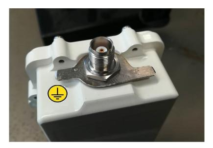
Besides the mains voltage safety, proper grounding is essential also for the error free operation of radio links and the protection against over-voltages and lightning. Although SATEL Proof-TR4 / -TR incorporates a robust internal surge protection, the surge spikes and power transients caused by lightning, ESD or other electrical systems must be discharged to earth ground.
