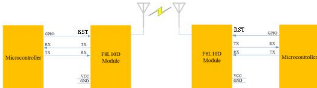
Figure 3-2 The UART convert to RF system
