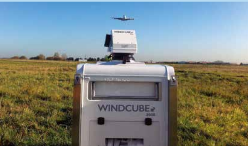
Windcube 200S deployed by Eurocontrol in the frame of RECAT operational deployment in CDG Airport
